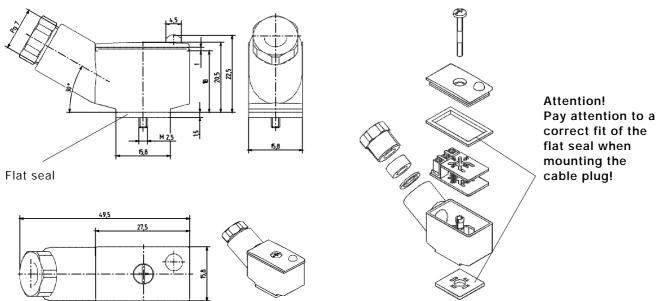
Cable plug type 2506 (pin assignment acc. DIN 43650, Form C)
